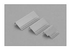
Upper ground return shield could be pre-instslled to the female connectors, the lower shields are provided and assembled separately after installing of the connectors onto the printed circuit board as required. Both the upper and lower shielding covers could bd ordered sepatately.
