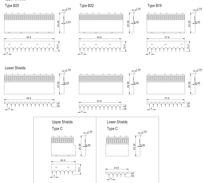
Dimensions shown are for reference purpose only, All dimensions are in millimeters unless otherwise specified.
