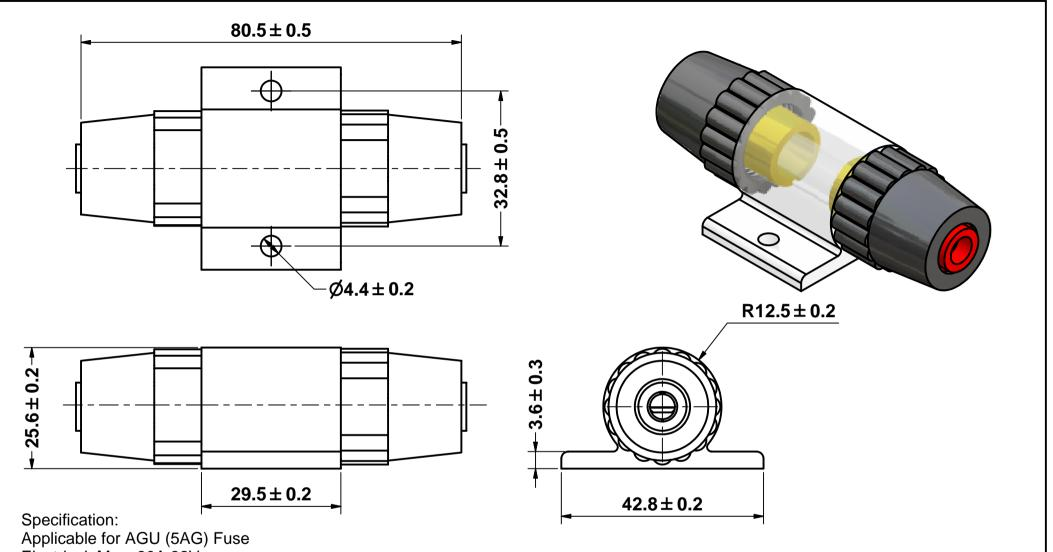
Electrical: Max. 80A 32V Insulation Body:Clear P.C
