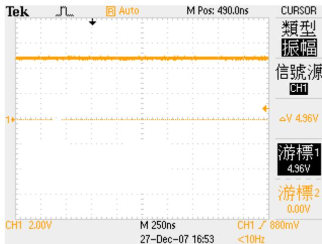
Fig.3 The voltage waveform at CAP
