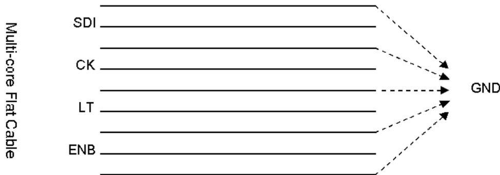
Fig.4 Separating the transmission lines with GND wires
